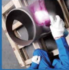
PT Inspection 渗透探伤
